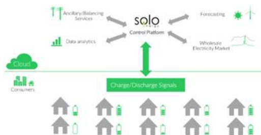
Solo Energy solution scheme
